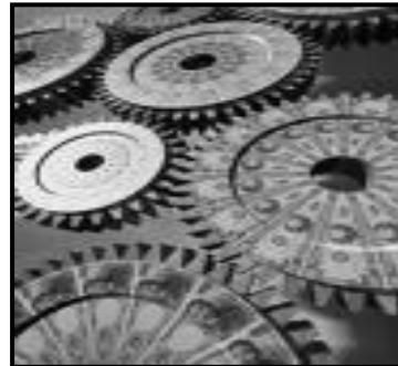
The meshing cogs prevent the slipping that occurs in a belt system.
